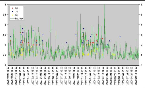
Fig. 5 Mean comfort for operational simulation of options A, B, and C of route 3 Genova-Peireos and maximum significant wave height for the control route
