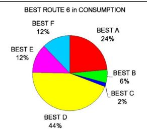
Fig. 8 Frequency of times when the six options of route 6 (Larnaca-Cagliari) are best in bunker consumption
