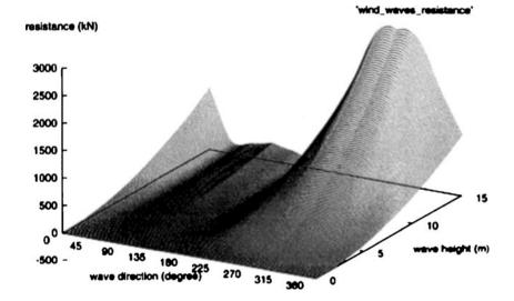
**Fig. 2** Example of added resistance to ship movement due to wind-waves (Hoffschildt et al. 1999)
