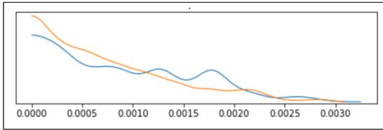
Fig. 9. Posterior pdf of leakage on the connection hose.
